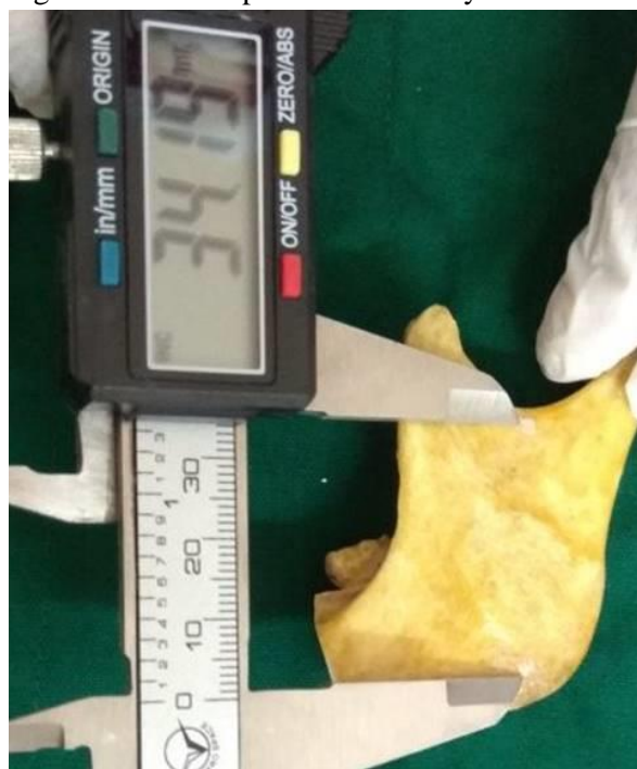
Figure - 3: Linear measurement at site A using digital vernier calipers on human dry mandible.
